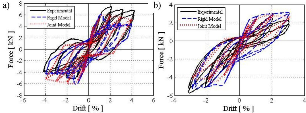
Figure 2: Comparison of the “rigid model” and “joint model” to experimental data for the a) interior subassemblage and b) exterior subassemblage.
