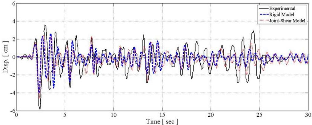
Figure 3: 3<sup>rd</sup> story displacement comparing one-third scale experimental data with “rigid model” and “joint-shear model” using the Taft motion at PGA of 0.30g.
