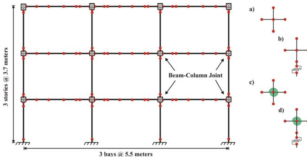
Figure 1: OpenSees two-dimensional model of full scale building with four different combinations of the joint and column spring details: a) rigid, b) shear, c) joint, d) joint-shear. Beam and column section details are found in (Bracci et al. 1992a).
