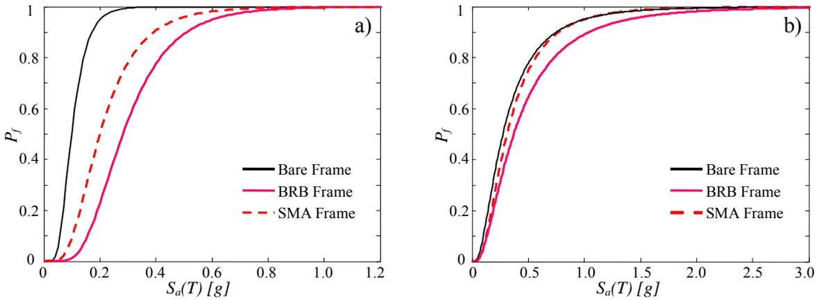
Figure 3-3 Fragility Curves Comparison at the Moderate Damage Level for: a) Structural Components at the 1<sup>st</sup> story, b) Non Structural Acceleration Sensitive Components at the 3<sup>rd</sup> story.
