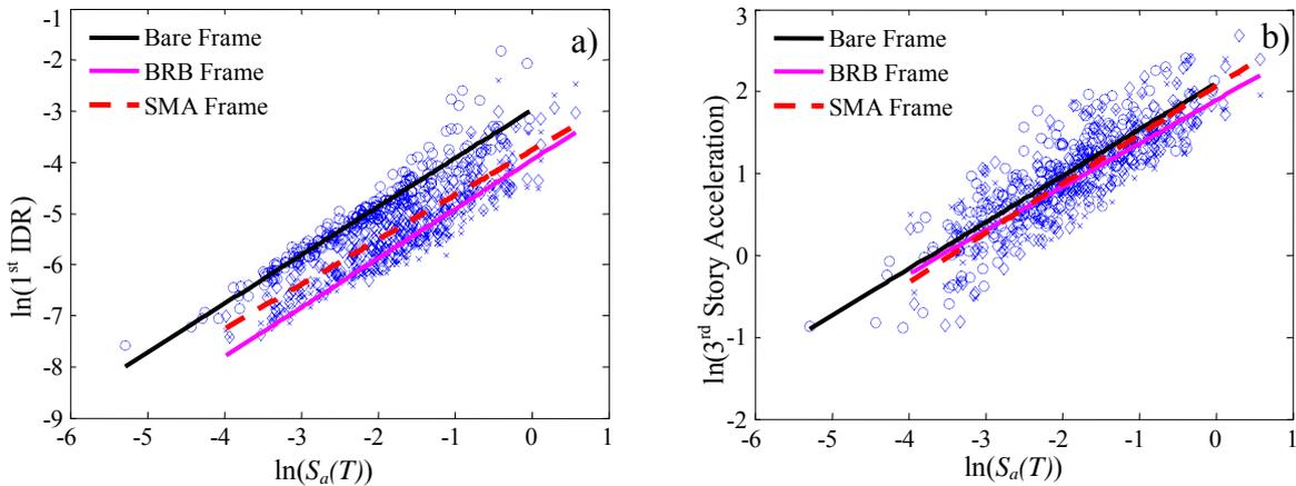
Figure 3-2 Probabilistic Seismic Demand Model Comparison for: a) Interstory drift at the 1<sup>st</sup> story b) Story Acceleration at the 3<sup>rd</sup> story.
