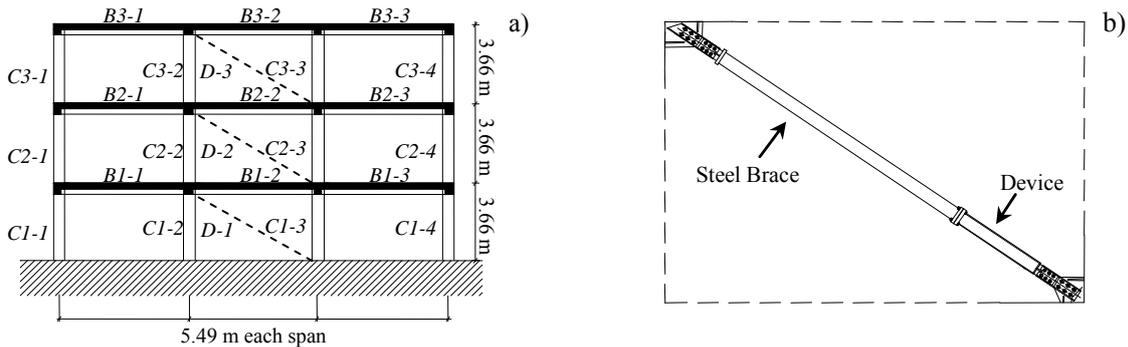
Figure 3-1 a) General layout of the structure and braces arrangement (adopted from [8]), b) Brace configuration.
