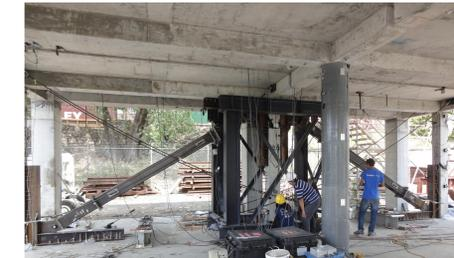
Responses of the SMA braced frame and the unretrofitted frame to the shaker excitation were investigated by analyzing floor displacement data. Input excitations included an El Centro ground motion record with amplitudes ranging from 1" to 12" shaker mass displacements and pulses ranging from 4" to 26".
