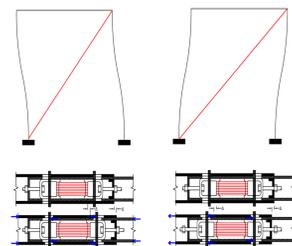
The braces were designed and assembled such that the SMA component remained in tension while the two HSS tubes were pulled apart (brace in tension) or pushed together (brace in compression). This allowed for the use of slender SMA sections, which reduces the required amount of SMA material, relative to a tension-only bracing system.
