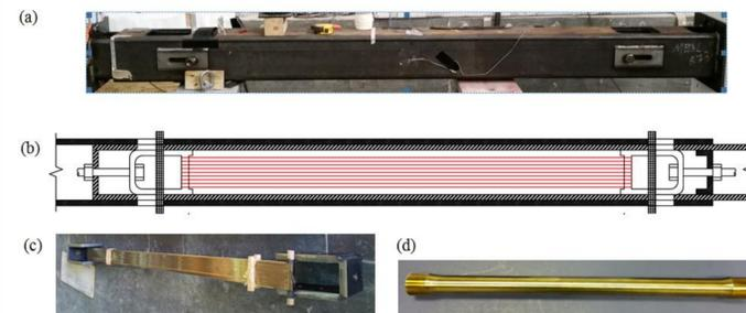
The brace device (a) consisted of an SMA component –wires (c) or rods (d)– housed inside two A500 steel hollow structural section (HSS) tubes, as seen in the section drawing (b).
