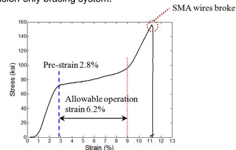
The stress vs. strain relationship of SMA wires under preliminary individual tension tests is shown above. The wires reached the forward transformation yield stress at 2.5% strain, entered the second strain hardening transformation at 9.0% strain, and eventually broke at 11.2% strain.
